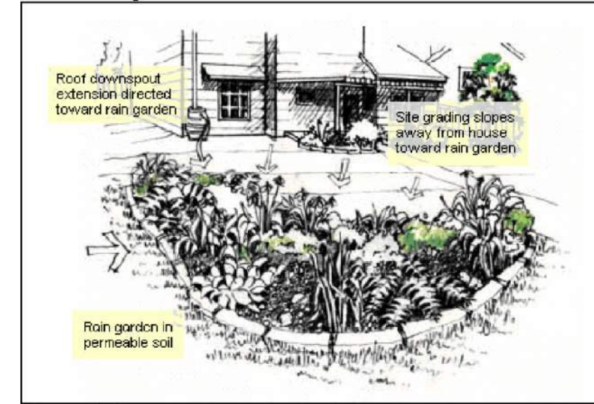
Figure 1: Layout of a typical rain garden
